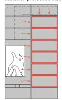
Technical box with radiation protection plate inserted
