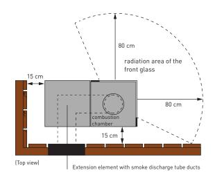
Extension elements, **through which smoke discharge tubes are fed** can be installed at a distance of at least 15 cm to **combustible elements** or walls (please observe the DIN of the smoke discharge tubes).
